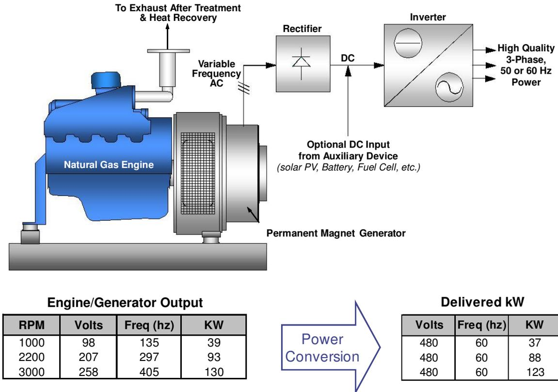
FIGURE 1. CONCEPTUAL DESIGN OF INVERTER-BASED ENGINE GENERATOR
