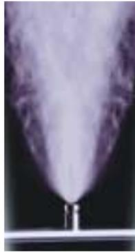
**Figure 3. Typical fog plume of MeeFog Nozzle. The high surface area of the billions of droplets permit rapid evaporation in even high humidity conditions.**
