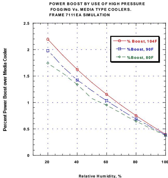
Figure 4. Power Boost by the use of High Pressure Fogging vs. Media Type Coolers
