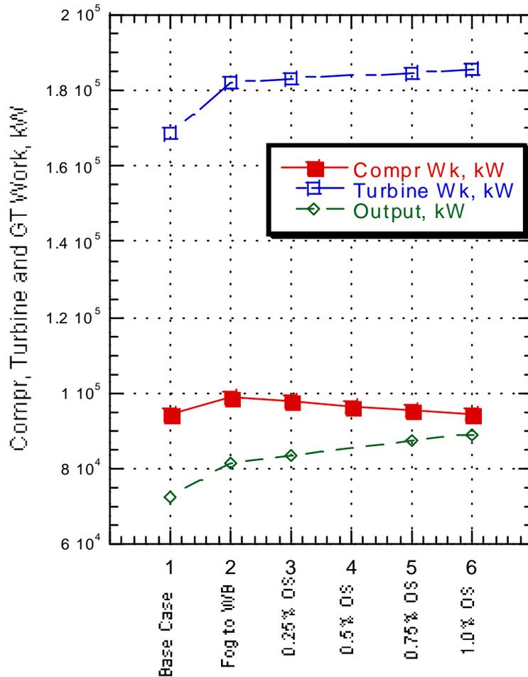
**Figure 5. Variation of Compressor and Turbine Work from Base case (1) through Saturation (Case 2) and overspray upto 1% Overspray. The fog intercooling of the compressor causes the compressor work to decrease as shown while the turbine work increases, resulting in net increase in output. Overspray capability can be very profitable during peak periods when peak rates are very high.**
